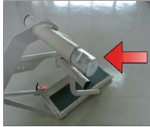
Get the Extension Bolt by spanner 24mm.
