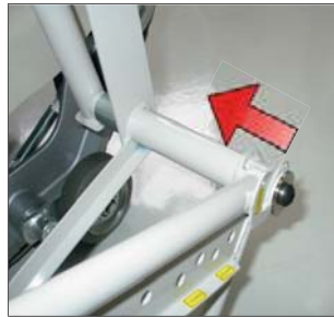
Slide in the Shoe Attachment until it touches the Extention Pipe.
